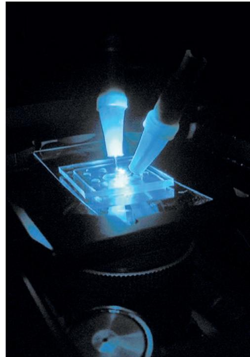
Microfluidic chip with electrical contacts for sorting DNA molecules. Image credits: Experimental Biophysics, Bielefeld University.
