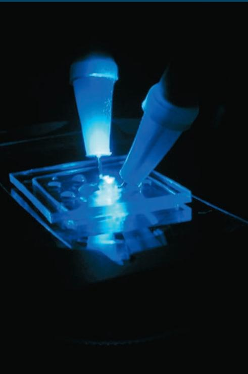
*Microfluidic chip with electrical contacts for sorting DNA molecules.
